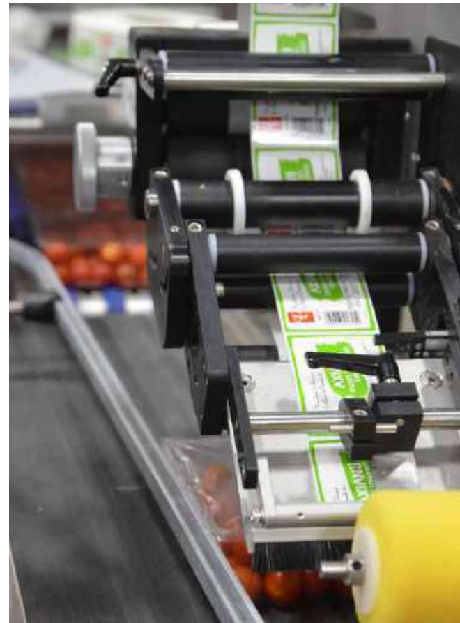
A closeup of the high-speed label applicator just outside of the Top Load Modular Cell system primed to label finished packs.
