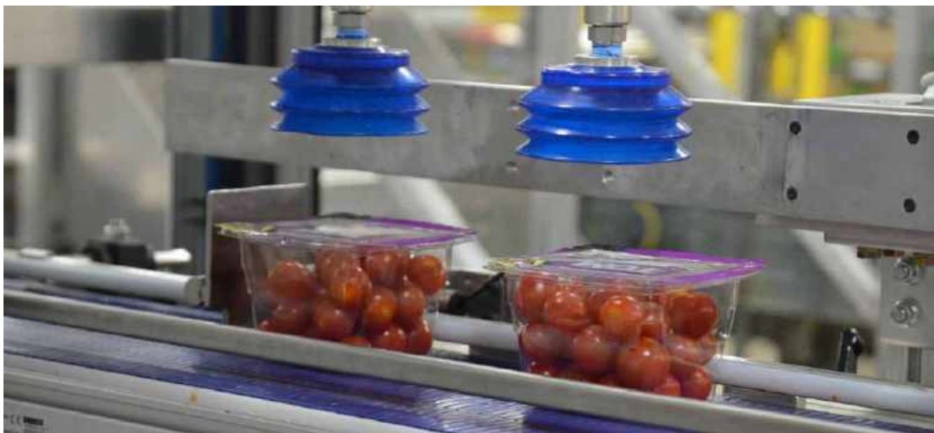
The Top Load Modular Cell system supplied to the Delta plant by EndFlex employs two soft-grip suction grippers on the end of the robotic arms to ensure swift and gentle handling and packaging of the top-sealed plastic tomato pints, with the system's modular design also offering the option of adding up to eight more robotic arms into the workcell to increase throughput rates.
