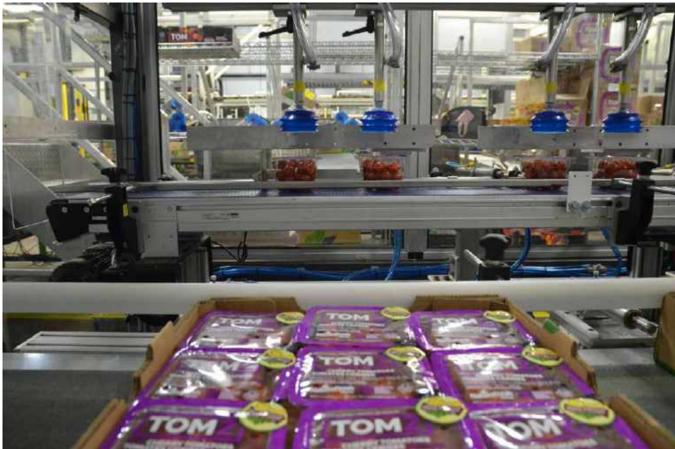
Corrugated shipping containers filled with plastic pints of TOMZ brand specialty tomatoes packed inside the EndFlex Top Load Modular Cell systems (background) await their turn to be moved to the plant's shipping area for prompt delivery to customers.
