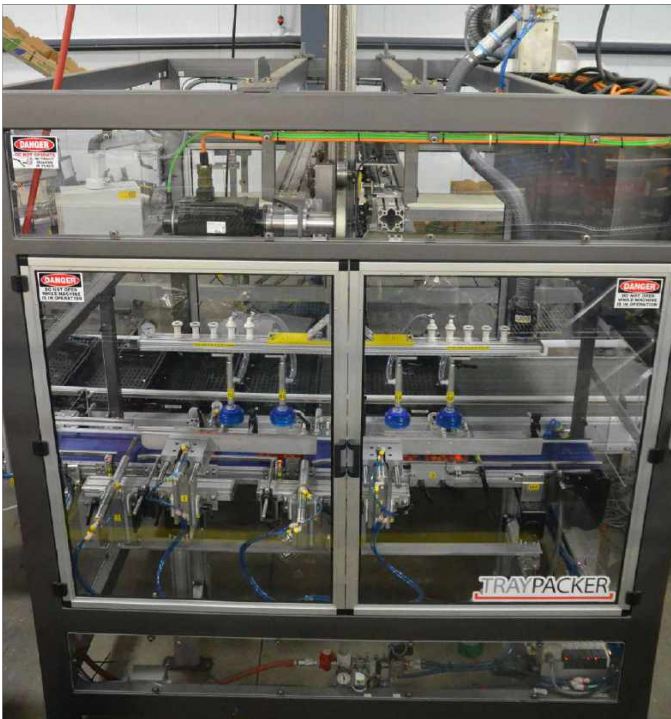
Manufactured by EndFlex LLC in Miami, Fla., the Top Load Modular Cell system is a fully-automtic workcell that enables the Delta plant to pack its fresh premium tomatoes inside plastic trays or bowls at robust throughput rates of about 60 packs per minute.
